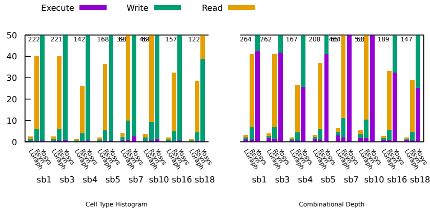
Figure 4: LGraph has a much smaller read and write overhead, since it uses memory maps to prevent parsing. Traversing a netlist in LGraph is as fast as RSyn and is faster than Yosys, in particular for ordered traversal.
